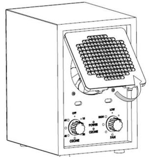
Then take front grill away in parallel. Reinstall After clean, first step put top latch of front grill in front panel slot then turn over down and push bottom latch of front grill in front parallel slot.
