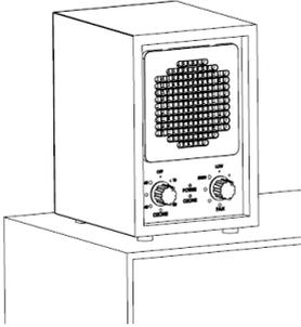
In order to maximize the purification function, the unit should be placed as higher as possible, or base something in the unit bottom to make the air blast window tilting upward so as to better oxidize and purify the floating bacteria and smog pollutants. A ceiling fan can also aid in purification of the unit. The air purifier is most effective when placed in a position that allows the anion & ozone mixed evenly and thoroughly with the polluted air.
