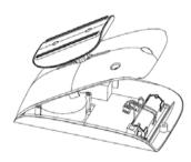
2. With the front remaining tilted up, slide the lower half of the case back and up until it is free.
