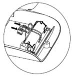
3. Disconnect the two leads of the Ozone Plate Assembly from the main circuit board.
