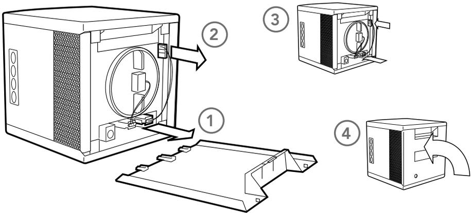
Remove the back panel and unplug the power connector to the purification plate. Remove the purification plate from its slot. Reverse order to replace plate.
