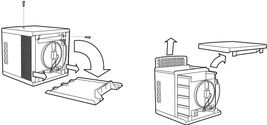
Slide out the side grills. Remove the 2 screws behind the back panel and the one on top. The top will pull away and front grill will slide up and out. Now you can completely clean the fan and the inside of your ecobox.
