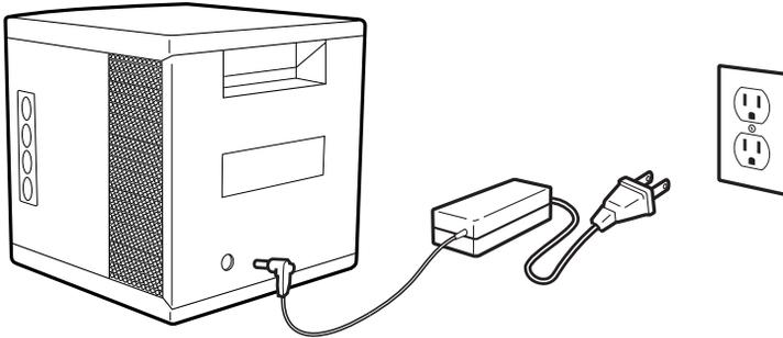
Plug power supply into the back of the ecobox and into a standard wall outlet.
