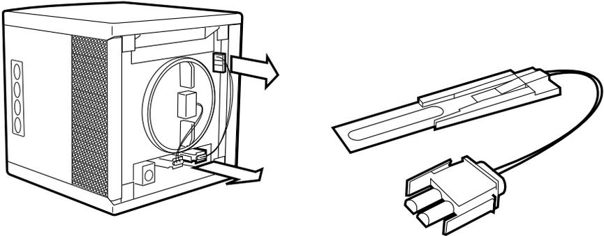
Remove the purification plate from its slot. Clean plate by wiping with a cotton swab dipped in denatured alcohol. Allow plate to dry completely before reinstalling.
