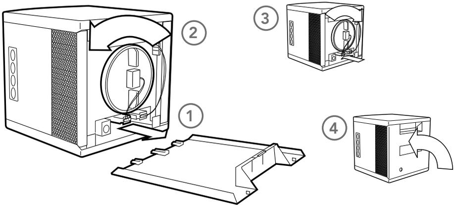
Remove the back panel and unplug the power connector to the RCI cell.
